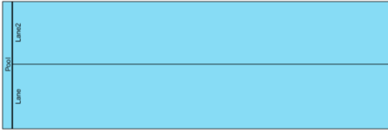
Horizontal pool that contains two lanes
